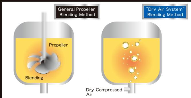
Sunoco uses its “dry-air” method in Japan to blend its products by blowing dry-air from the bottom of the blending tank. This method is well suited for refrigeration oils, where impurities are strictly forbidden. In the usual blending method, a propeller is used and lubricants or water may become detached from mechanical parts and mix with the oil. The “dry-air” method minimizes this risk.
